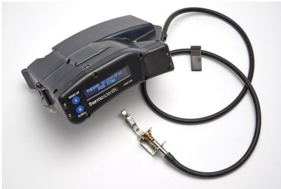
Figure 6 - Miner safety product resulting from commercialization of the Personal Dust Monitor technology developed at NIOSH [11].
