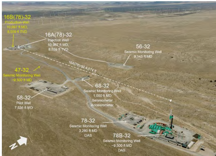
Figure 1. Aerial view of the Utah FORGE site. Wells denoted in white have been drilled; wells in yellow will be drilled in the future. The dashed line is the surface projection of well 16A(78)-32 drilled at 65° to the vertical on an azimuth of 105°.
