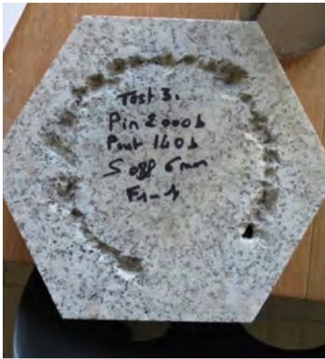
Figure 3. Example of a slotted Sidobre granite rock specimen.
