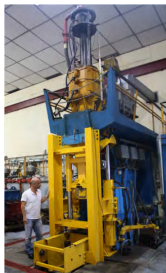
Figure 1. An experimental setup of ARMINES for vertical drilling, Pau.
