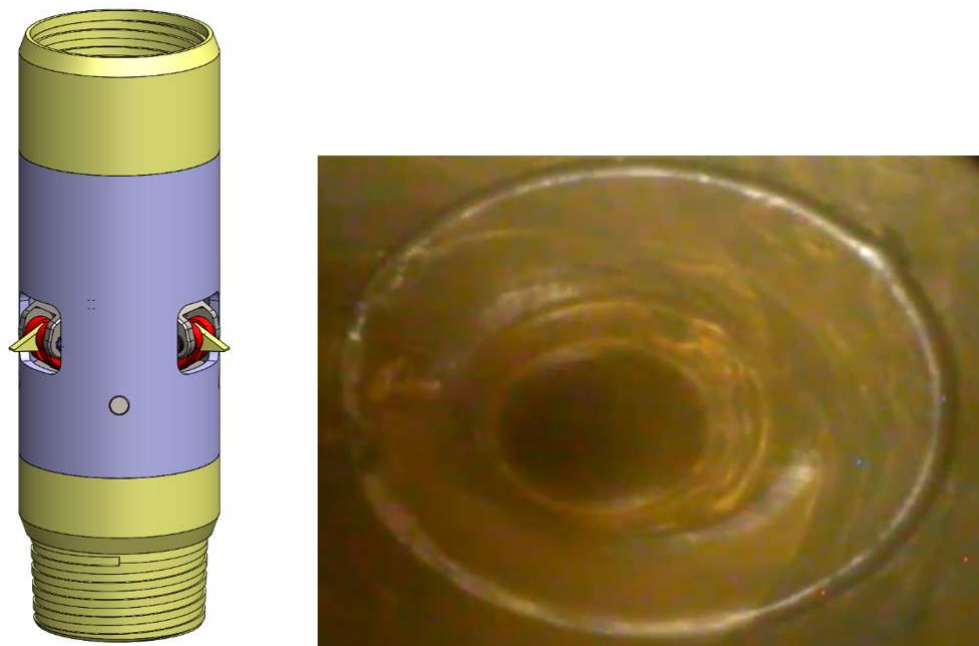
Figure 3. Left: The notching tool developed by Sandia National Laboratory. Right: An example of the notch engineered by the tool.
