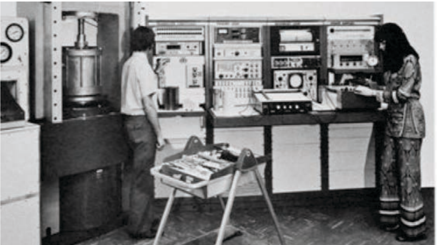
Dr. Ted Brown and Raquel Derrenberger, Senior Laboratory Technician, Rock Mechanics, with the servo-controlled rock testing machine.
