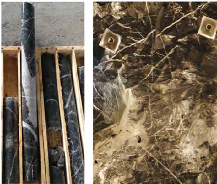
Figure 6a. Characterization of hydrothermal quartz veins commonly encountered in block caving of porphyry copper deposits (after Day, 2016).
