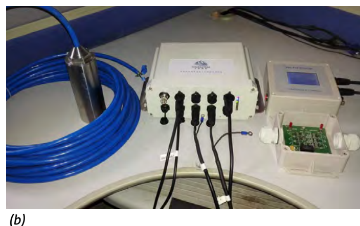
Figure 3. (a) An apparatus for distributed stress monitoring based on Fiber Bragg Grating technique. (b) The developed intelligent microseismicity system with the system sensibility of 2.2 microvolt and PTP with high accurate time clock are adopted.
