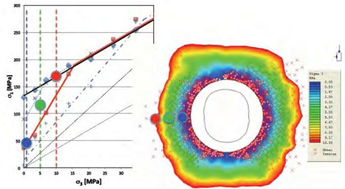
Figure 8. Right: Continuum model of tunnel showing yield locations (x and o) for  $k_0 = 0.5$  and confinement contours; Left: Illustration of three states at locations indicated by circles in principal stress space for marble (Figure 5).
