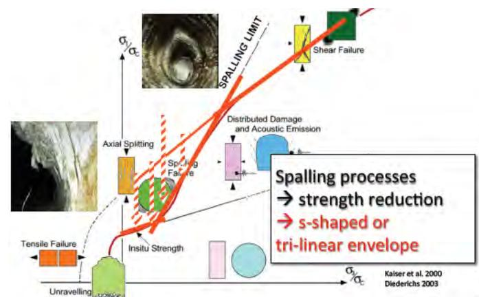
Figure 4. Principal stress space showing depressed failure envelope in low confinement range and related excavation failure processes: spalling, notching, and shear rupture.
