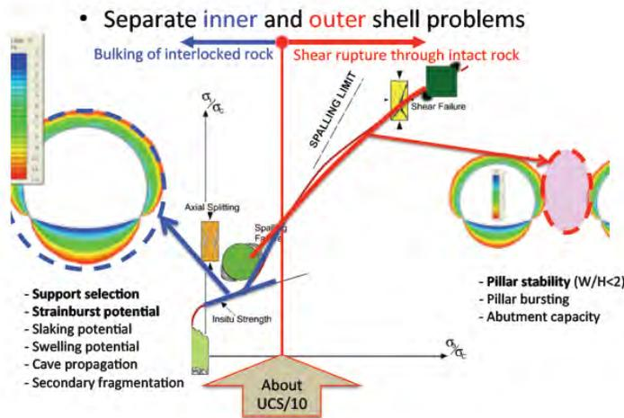
Figure 7. Zoning of stress space for inner and outer shell
