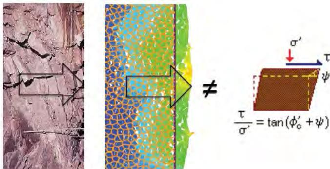
Figure 10. Unidirectional rock mass bulking due to stress-fracturing (left) reflected in Voronoi model (cartoon-like model in center) and non-representative dilation model (right).
