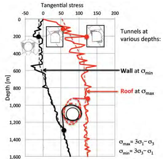
Figure 11. Example of mining-induced minimum and maximum tangential stress profiles for a circular tunnel in a tectonically strained environment. Also shown are various failure modes reflected by the behavior matrix of Figure 3.
