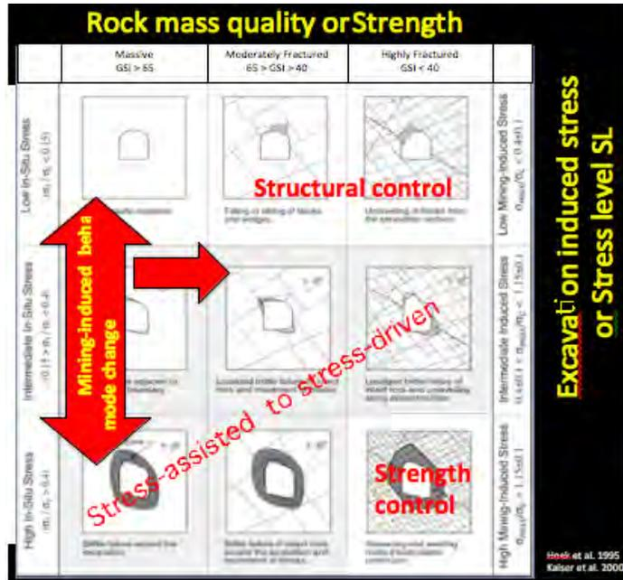
Figure 3. Excavation behavior matrix with indication of anticipated failure mode changes resulting from mining-induced stress-paths (after [ 3] and [ 8]).
