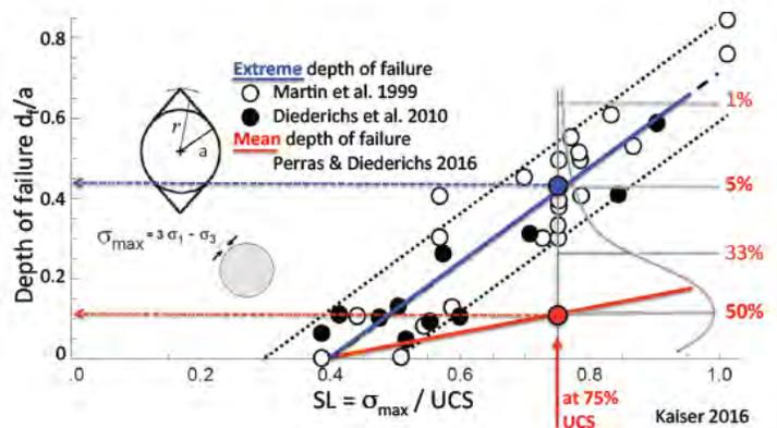
Figure 9. Depth of failure chart for extreme and mean conditions; also shown is an approximate frequency distribution at  $SL = 0.75$ ;  $a =$  tunnel radius.
