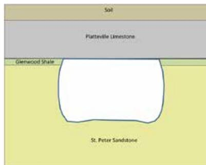
Figure 1. Geologic cross-section at the LRT station.
