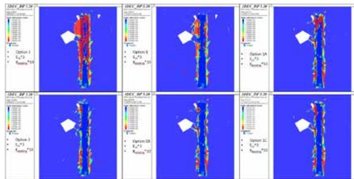
Figure 9. Predicted factor of safety against slip for the bedding plane at elevation 789: Option 1 model (upper left); Option 1' model (upper center); Option 1A model (upper right); Option 2 model (lower left); Option 1B model (lower center); and Option 1C model (lower right).
