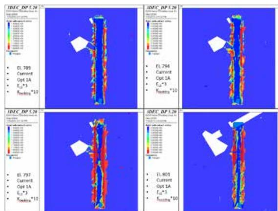
Figure 8. Predicted factor of safety against slip for the current station condition for the bedding planes at elevation 789 (upper left), 794 (upper right), 797 (lower left), and 801 (lower right).
