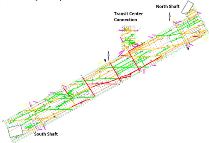
Figure 3. Platteville limestone joints mapped during construction.
