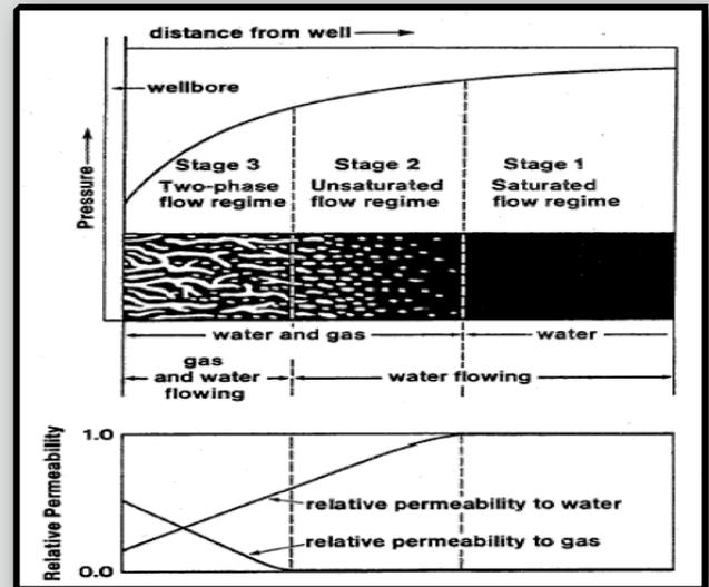
Figure 2: Three stages of coalbed gas production.
