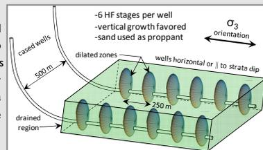
Figure 1: Multiple HF stages for shale gas stimulation.
