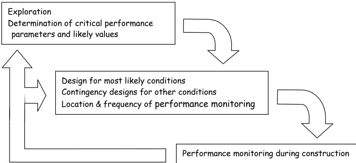
Figure 4. Observational method (feedback).
