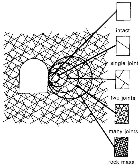
Figure 2. Concept of scale as it pertains to rock mass properties (from Hoek and Brown, 1981).
