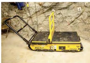
*Figure 10: The Track-O will move lead shielding to and from the lower Davis Campus*
