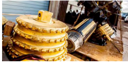
Figure 6: The team drills a bore hole 300 feet down and will back ream using the rig pictured here
