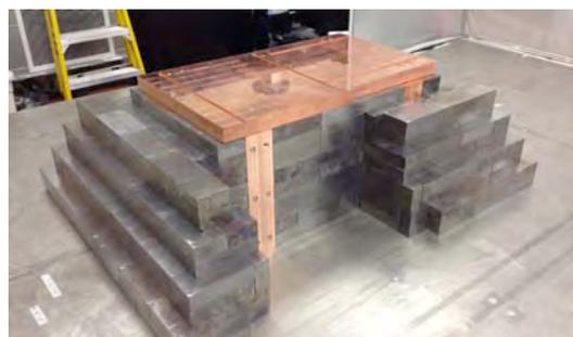
*Figure 6: Stacked lead bricks will help shield the sensitive MJD experiment*
