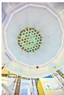
*Figure 4: White Teflon lines the interior of the LUX detector, to better gather faint signals of light that will be recorded by the photomultiplier tubes (center).*
