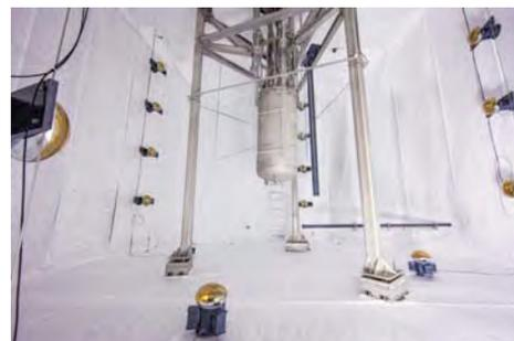
*Figure 3: The LUX dark matter detector suspended in its protective water tank. The detector is a titanium cryostat—that is, a vacuum thermos—that will keep xenon cool enough to remain a liquid, at about minus 150°F.*
