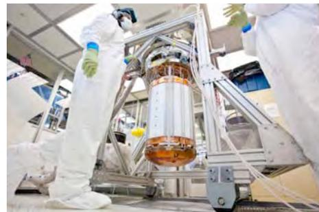
*Figure 2: LUX researchers, seen here in a clean room on the surface at the Sanford Lab, work on the interior of the detector before it is inserted into its titanium cryostat*
