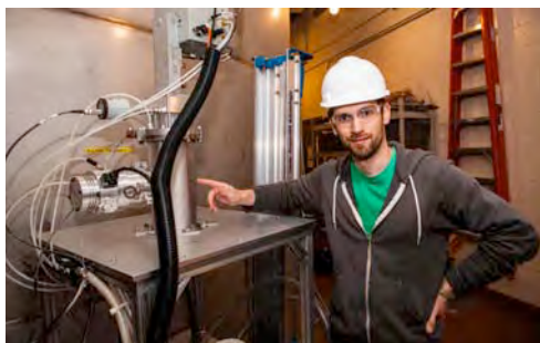
Figure 3: James Verbus points to the cylindrical neutron generator that the LUX team is assembling
