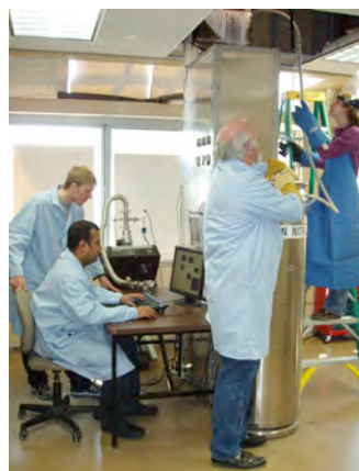
Figure 2: Four University of South Dakota grad students work on a cryogenic distillation column
