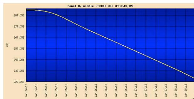
*Figure 2: Chart tracking the progress of cooling the LUX dark matter detector. Time was tracked on the horizontal axis (starting January 24), and temperature in Kelvin was tracked on the vertical axis*
