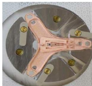
*Figure 6: Fused silica (glass) low mass front-end board, with electronics loaded, is mounted in a copper leaf spring*
