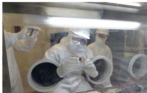
*Figure 5: Ryan Martin assembles a detector unit in the glovebox of the MAJORANA DEMONSTRATOR assembly room at the Davis Campus 4850 Level*
