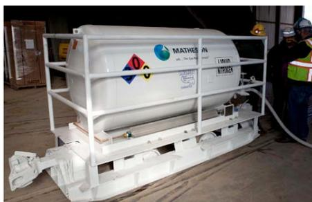
*Figure 7: New LN cart with liquid nitrogen to fill the LUX dark matter detector*
