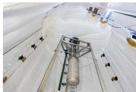
Figure 4: Small stream of water (left) filling the LUX water tank at the 4850 Level. The LUX detector (center) is 6 1/2' x 3' diameter. Photomultiplier tubes hang on the sides of the tank.
