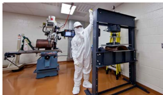
Figure 5: Machinist Randy Hughes uses a press to flatten one half of a copper cylinder that was electroformed at the MAJORANA Temporary Clean Room
