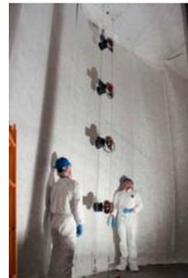
*Figure 5: LUX collaboration members John Bower (left) of Lawrence Livermore National Lab and Sergey Uvarov of UC Davis work on a string of four photomultipliers in the LUX tank*
