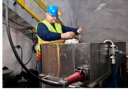
Figure 4: Ty Balmer of *Astro Pak* tests water during LUX water tank passivation
