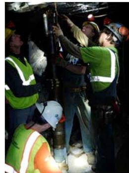
*Figure 1: GEOX™, SDSTA, and observers work together to position and assemble the hydraulic jacking system for 100-ton loading experiments. Standing from left: Rich Barry, Pat Kinghorn, and Luke Scott. Kevin Hachmeister, kneeling*
