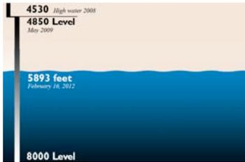
Figure 5: Progress of dewatering at Sanford Lab
