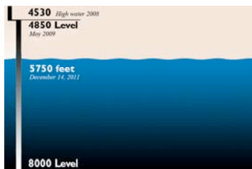
Figure 3: Progress of dewatering at Sanford Lab
