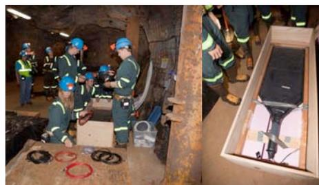
*Figure 16: (Left) The Davis-Bahcall Large Area Muon Detector Stack (DB-LAMDS) are cabled up by students Amanda Finley, Dan Pfeifle and Willie Hinker; (Right) Fermilab donated the three large scintillator detectors; data will be uploaded to the Quarknet e-lab site for use by schools around the country*
