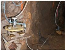
Figure 4: Wall mounted Budker style tiltmeter (foreground); Pedestal mounted Tevatron style tiltmeter (background)
