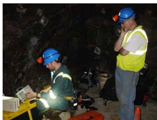
Figure 7: Matt Kogle and Steve Gabriel collect ultrasonic velocity data from rock bolts in the wall of the alcove
