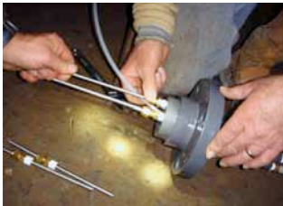
Figure 4: Extensometer made by Geokon, Inc.
